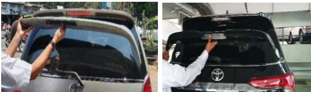
Figure 4 Product prototyping of car spoiler using rattan fiber composite
