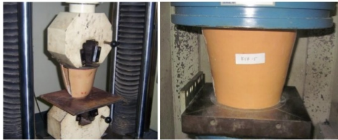
Figure 4. Compressive failure testing of socket product
