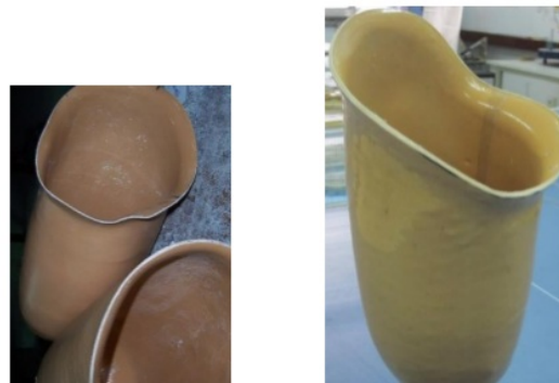
Figure 3. Socket product made from bamboo composites material
