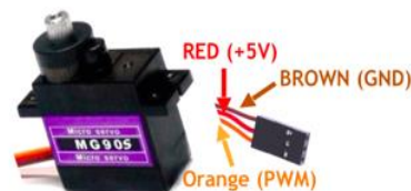
Figure 4. MG90S Servo Motor and Pinout
