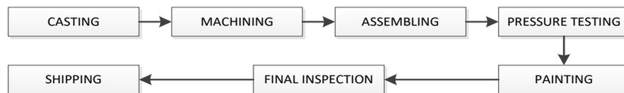
**Figure 1.** Valve production process
