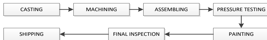
Figure 1. Valve production process
