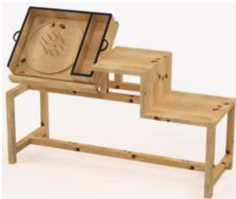
Figure 10. Helper tool to separate and pack spoons
