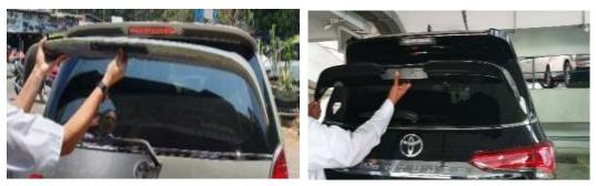
Figure 4 Product prototyping of car spoiler using rattan fiber composite
