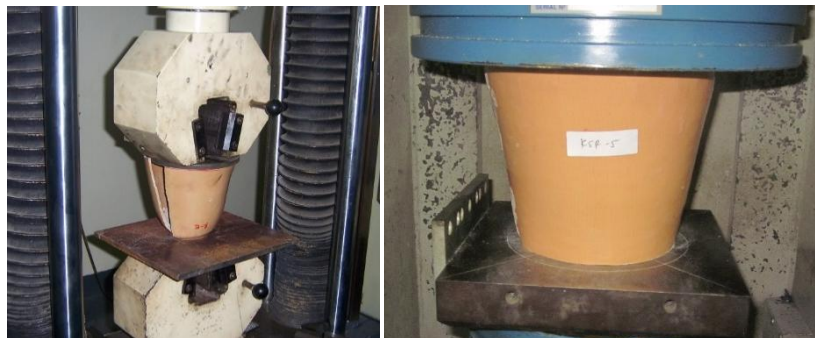
Figure 4. Compressive failure testing of socket product
