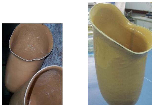
Figure 3. Socket product made from bamboo composites material
