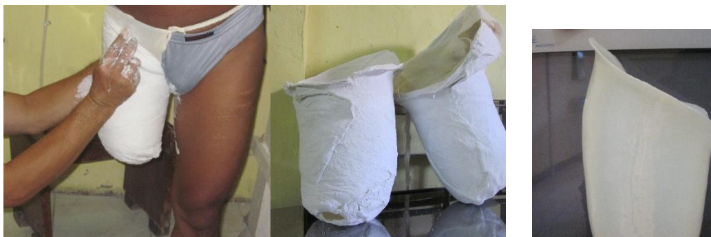
Figure 1. Manufacturing of negative mold of socket product
