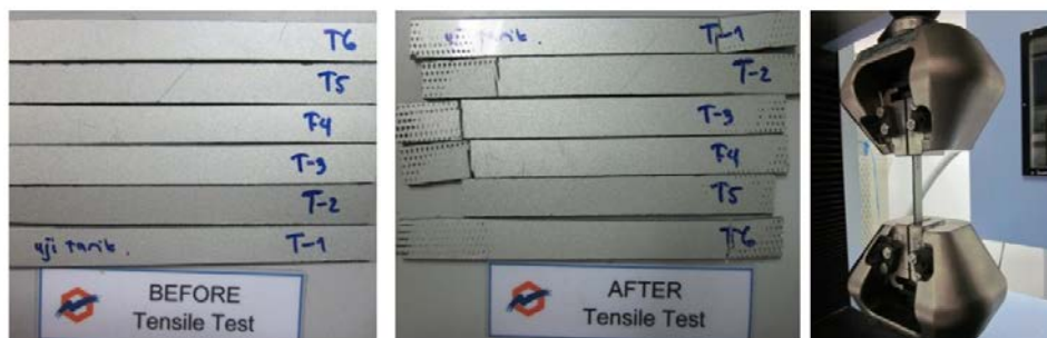
Figure 3. Sample test of car spoilers made from ABS plastic material and universal testing
