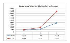
Figure 3. Comparison of BCube and DCell Topology Performance
