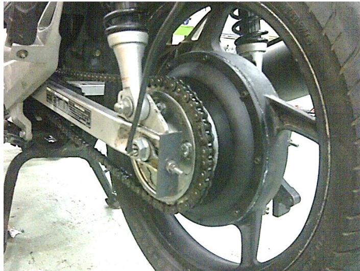
Figure 8. Final Assembly of Hybrid Electric Motorcycle
