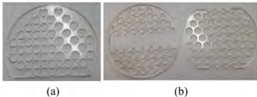
Fig. 2 Design of heat exchanger baffles. (a) triangular pattern 30^\circ - single segmental baffle, (b) rotated triangular 60^\circ - double segmental baffle
