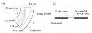
Fig. 1 Schematic of fully self-contained implantable artificial cochlea<sup>(7)</sup>; (a) top view and (b) cross sectional view at AB of (a).
