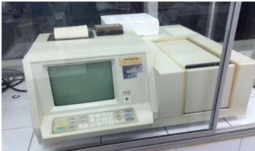
Uv-vis Spechtrphotometer Double Beam Hitachi Japan, model – 2000
