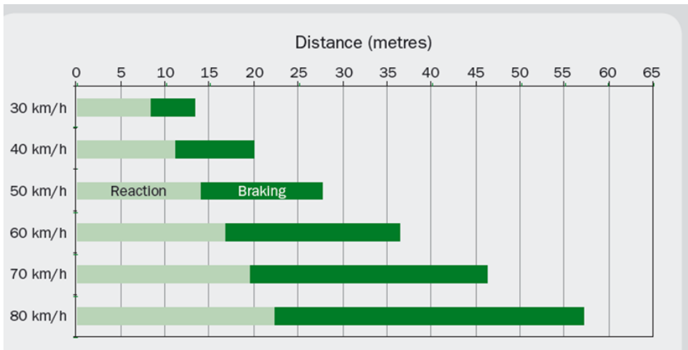
Figure 2 Effect of Vehicular Speeds on Stopping Distance Source: OECD/ECMT Transport Research Centre (2006)
