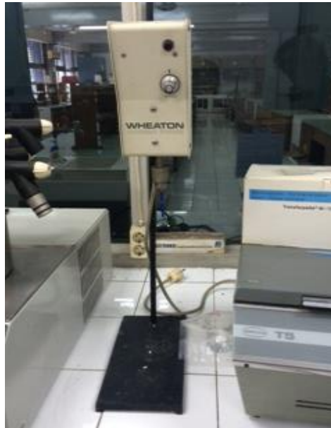
Tissue Grinder (Homogenizer) Wheaton Science, Millville, NJ-USA.
