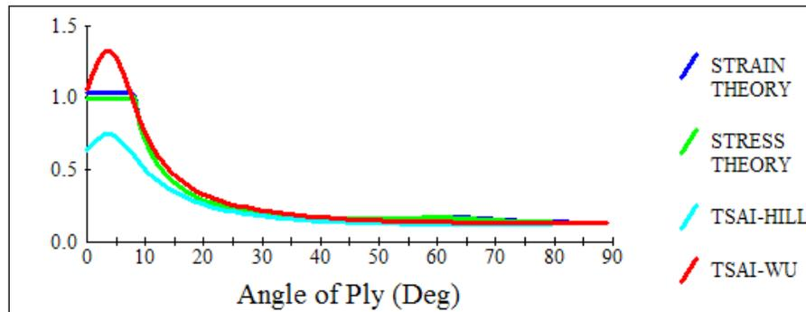
**Figure 1.** Strength Ratio (SR) of RFRECM
