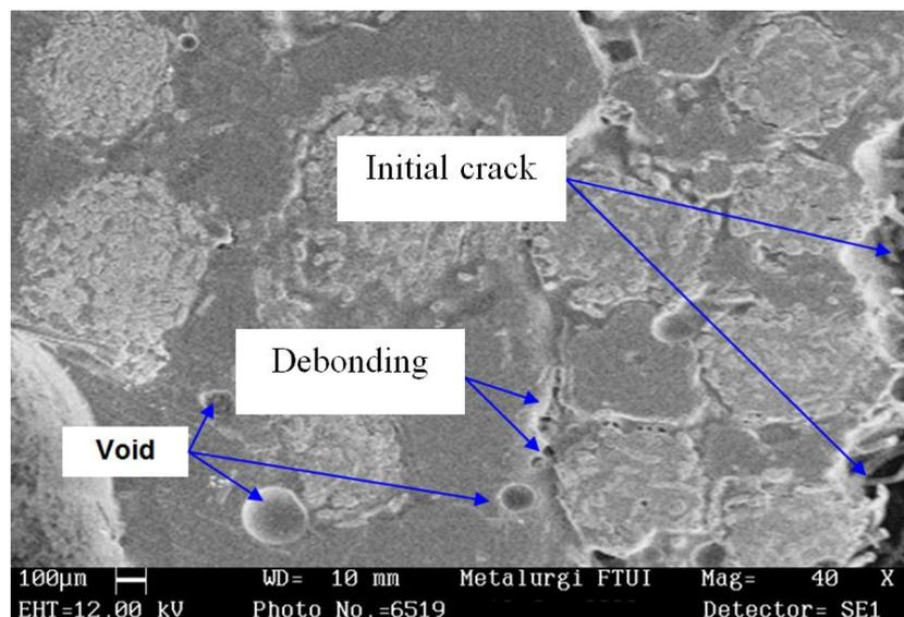
**Figure 5.** Morphological analysis of RFRECM by SEM
