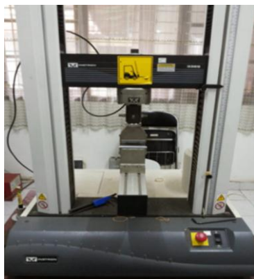
Fig. 4. Tensile Specimen Test of the BSRECM
