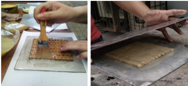
Fig. 3. Fabrication of the BSRECM
