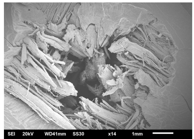
Fig. 9. SEM Result of 0^0/0^0/0^0 BSRECM Laminate after Ballistic Test
