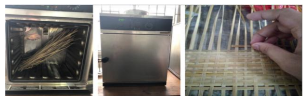
Fig. 2. Bamboo Strips Drying Process at a Temperature of 40^0\text{C}
