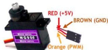
Figure 4. MG90S Servo Motor and Pinout
