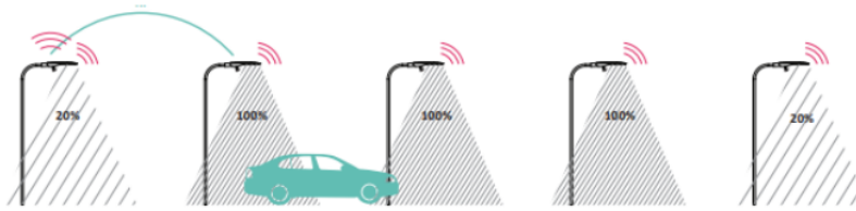
Figure 1. Smart Street Lighting Illustration
