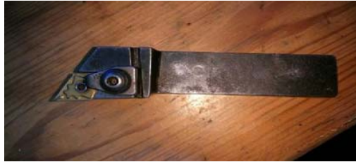
Figure 1. Carbide dan tool holder VMDJNR-2020-15 Table.1 The chemical composition of Steel AISI 4340
