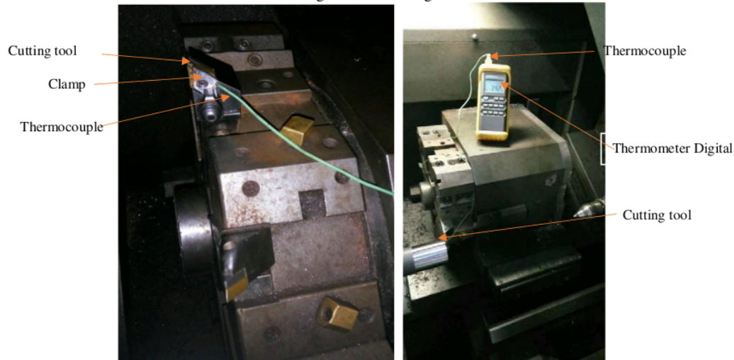
Figure 7. Clamp circuit, cutting tool and Testing Tool
