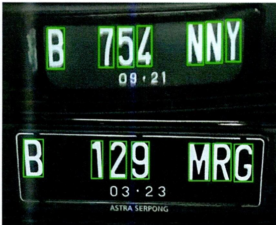
Fig. 4. Segmentation results of the detected license plate
