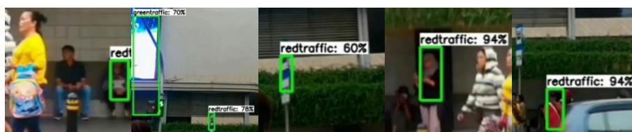
Figure 9. The Object Detection Result Which is Mismatch With The Pedestrian Traffic Light
