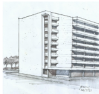
Figure 6. The eight-storey East-West side of the eight-storey Building M is made massive. The opening is only in the corridor. Dominant opening in North-South.
