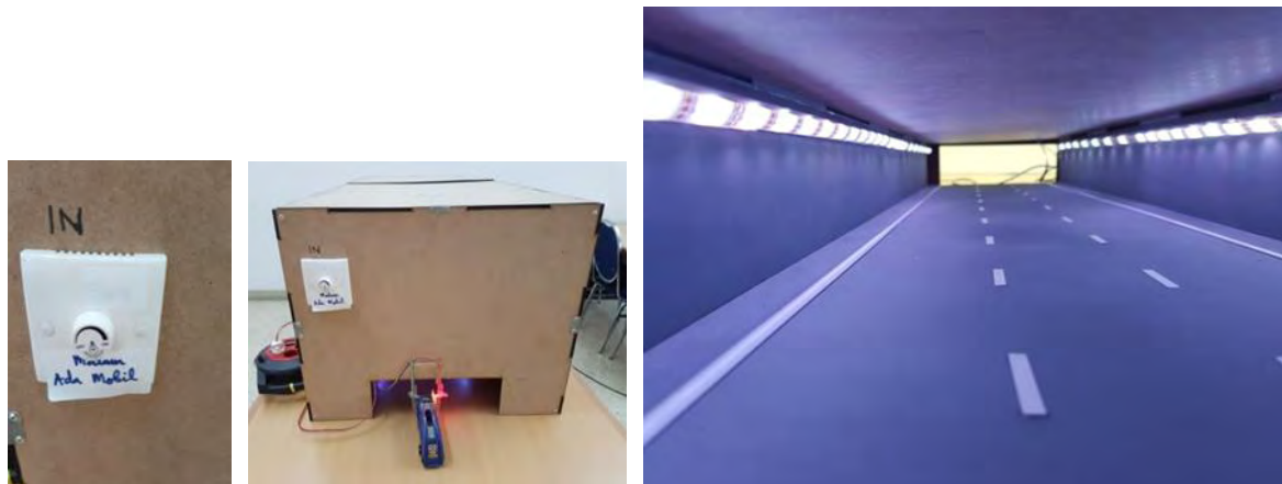
Fig.8 Realization of the tunnel lighting model when a car pass through
