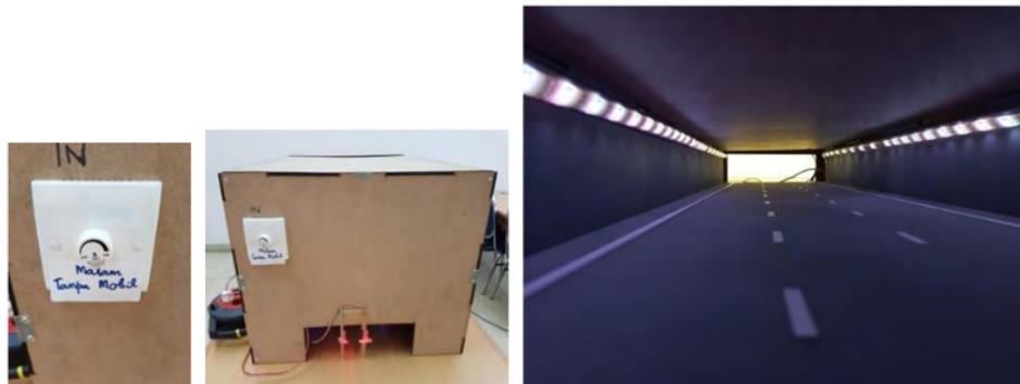
Fig. 7 Realization of the tunnel lighting model when no car pass through
