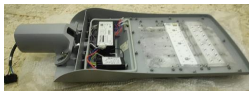
Figure 3. Position LED Drivers in Lamp Housing
