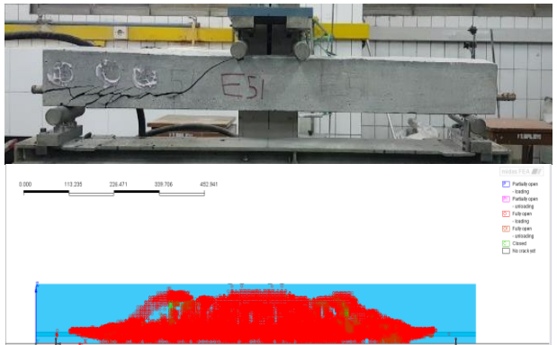
Fig. 9. Failure and Cracking Pattern of Beam E31
