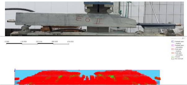
Fig. 16. Failure and Cracking Pattern of Beam E62
