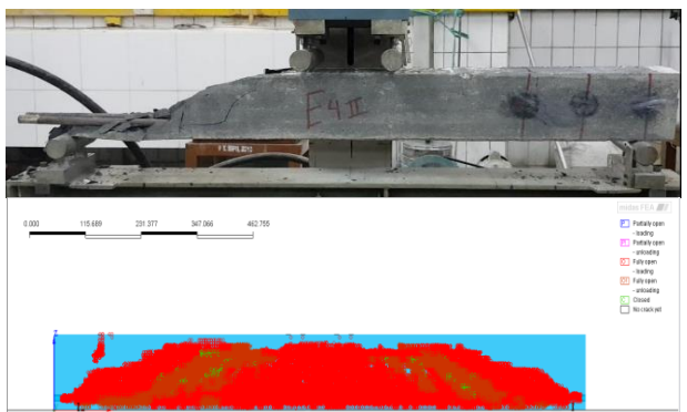
Fig. 11. Failure and Cracking Pattern of Beam E41
