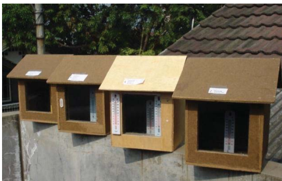
Photo 2. Mockups with a model home which has a glass window placed in an open space facing east, illuminated by the sunlight, ready to be used for data retrieval temperature indicated on the thermometer mercury at each hour from 09.00 AM until 16.00PM, for approximately one month (30 days).
