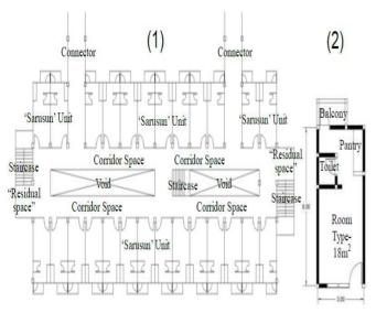
Fig. 5 (1) 2<sup>nd</sup> to 5<sup>th</sup> Floor plan block "A" building; (2) 'Sarusun' unit floor plan. Source: Private document, May 09, 2016
