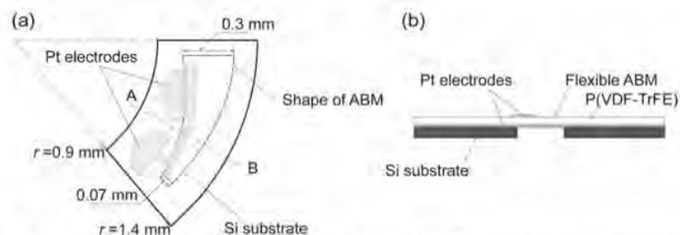
Fig. 1 Schematic of fully self-contained implantable artificial cochlea<sup>(7)</sup>; (a) top view and (b) cross sectional view at AB of (a).
