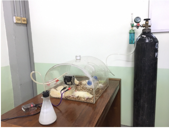
Chamber hypoxia, Soda lime, Tabung gas
